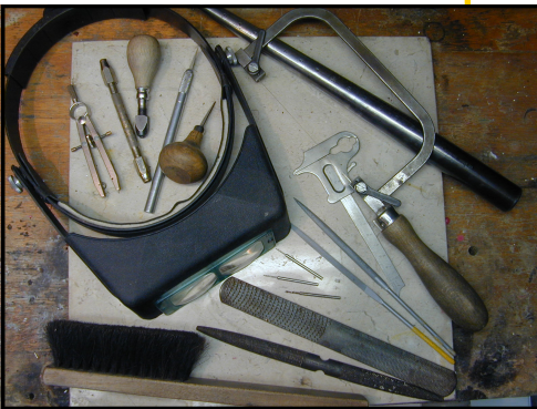
Larry Seiger’s tools (clockwise from top right): Ring mandrel, jewelers saw frame, millimeter gauge, needle files, small drill bits, coarse files, bench brush, magnifiers, compass, pin vise, millgrain holder, exacto knife and graver. Visit LSHancock Designs’ website at http://www.lshancock.com .
